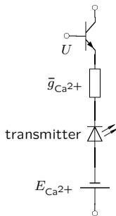
**Fig. 1.16.** Equivalent circuit for the calcium-controlled transmitter release (indicated by the arrows of the LED)
