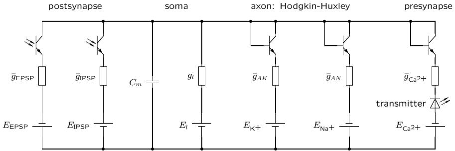
**Fig. 1.21.** Equivalent circuit for a neural point model
