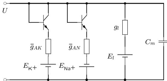
**Fig. 1.14.** Equivalent circuit for the Hodgkin-Huxley equations (1.25, 1.27–1.29)
